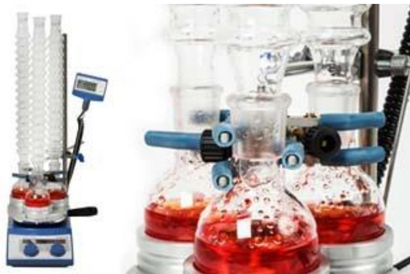
Driven by concern over numerous lab flooding incidents in their synthetic chemistry labs at both undergraduate and postgraduate levels from the use of Liebig water condensers, TU Dublin were drawn to evaluate Condensyn waterless condensers.
